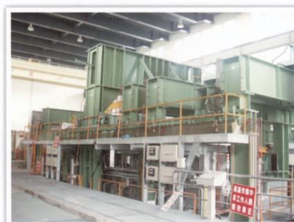
Beam, column composite fire test furnace
