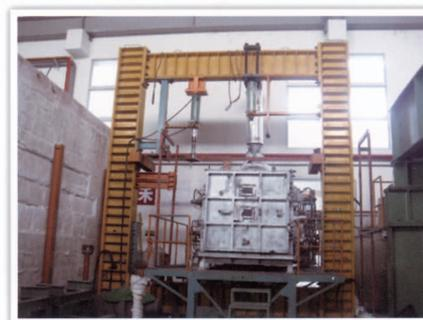
Small-scale fire test furnace
