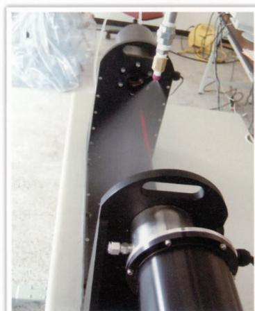
MALVERN Laser Diffraction Particle Size Analyzer
