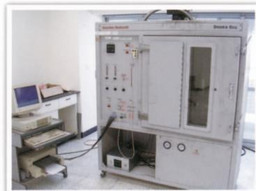
Test device for smoke concentration generated by solid materials
