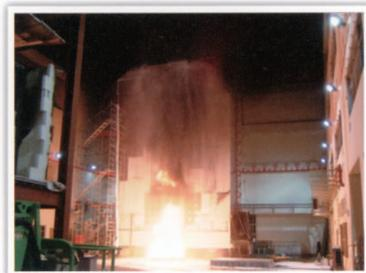
Fire-fighting test of foam sprinkler head
