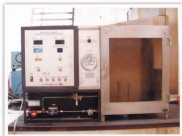
45° test device for flammability of thin materials
